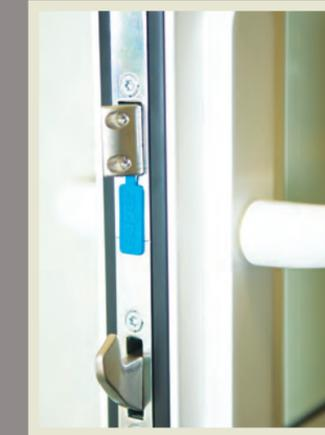
Sliding patio doors have anti-lift devices to prevent the lifting and removal of the sliding panes, and interlocking stiles to restrict the doors from being prised apart. The locking mechanism consists of 6 centre hooks operating on a stainless steel faceplate providing strength and a long lasting finish. The lock contains an anti-slam device meaning that you are unable to inadvertently shut the door with the hooks in the "locked" position and cause damage to the faceplate.
